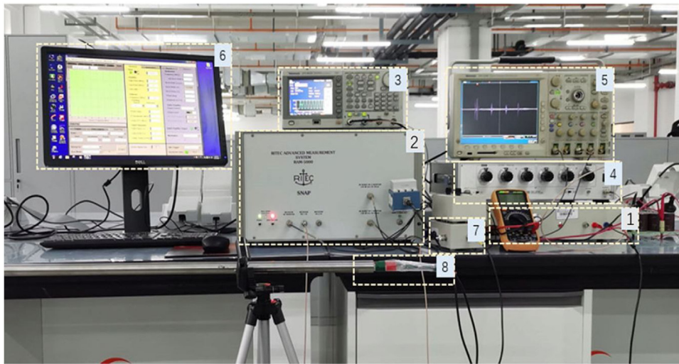
Fig. 6. Experiment setup for pipe inspection with the plug-in PPEM GW EMAT.
