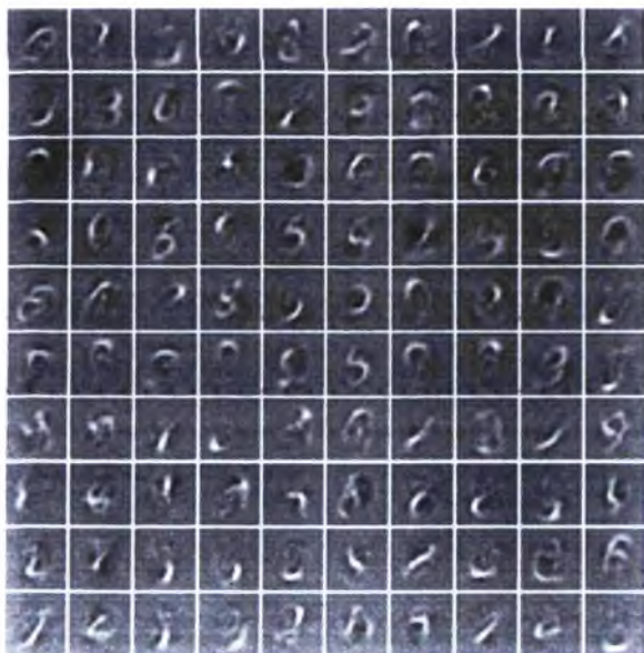
Figure 8.5. Results of training the 1 st autoencoder to compress the input image
