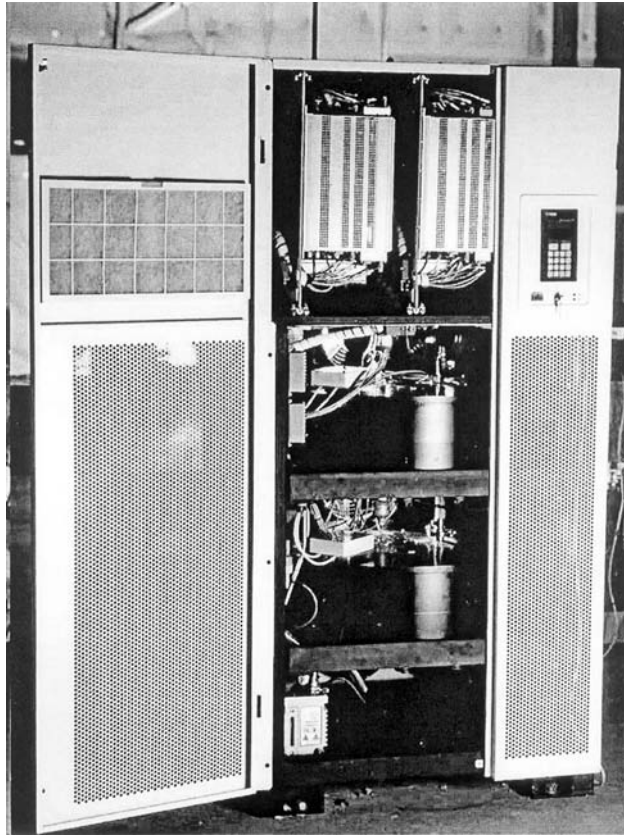
Fig. 6.61 A 240 kW flywheel system. (Courtesy of Active Power Inc., USA.)
