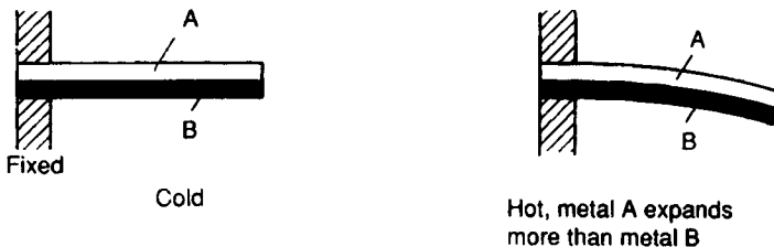
Figure 1.21 Bimetallic strip
